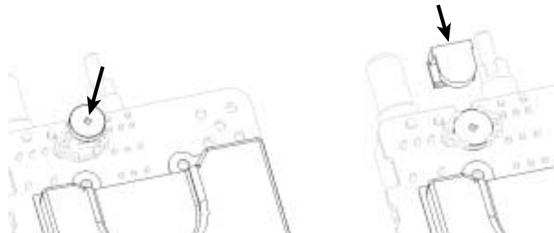
Figure 40. Reassemble the Backup Battery
